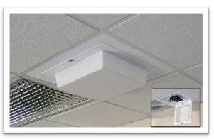
It is also important to note that the AP-92/93, AP-105, and AP-130 series of 802.11n access points are uniquely designed, combining form and function in a small, efficient, tool-less mountable package that discretely blends into the environment where it is deployed. Aruba 802.11n access points models support above ceiling tile (UL-2043 listed / plenum-rated), wall, or tool-less ceiling mounting to a variety of ceiling tile rail types.
